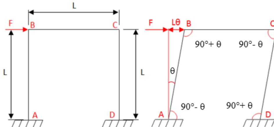
**Figure 1.** (a) Schematic model for a frame under application of load. (b) Collapse mechanism. Source: own authorship (2021).
